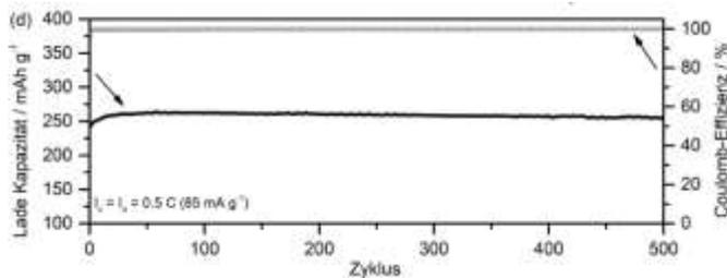
Electrochemical performance of the anatase TiO<sub>2</sub>/C in a lithium ion cell
