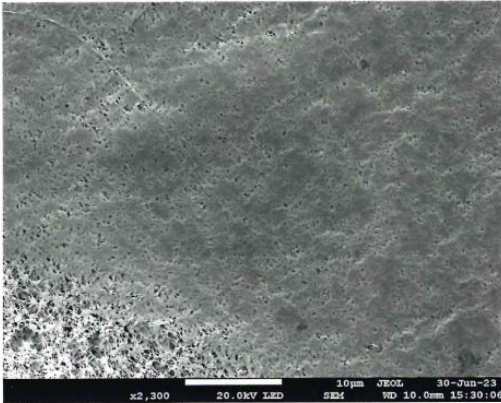
Figure 1: The SEM image shows that gold sputter-deposited on the PTFE membrane forms a continuous film, which features mostly individual offices of the pores (dark spots).
