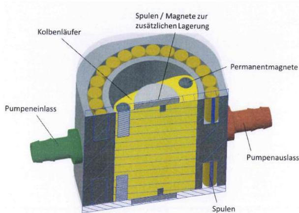
over the life of the product and bypass interactions between the fluid and the seals. Due to the elimination of the sealing joints, the new technology is particularly suitable for use as a blood pump. Conventional blood pumps have considerable problems with possible blood clotting due to a lack of tightness, which can lead to thrombus formation. Blood deposits resulting from seals can also cause the pump to fail.
