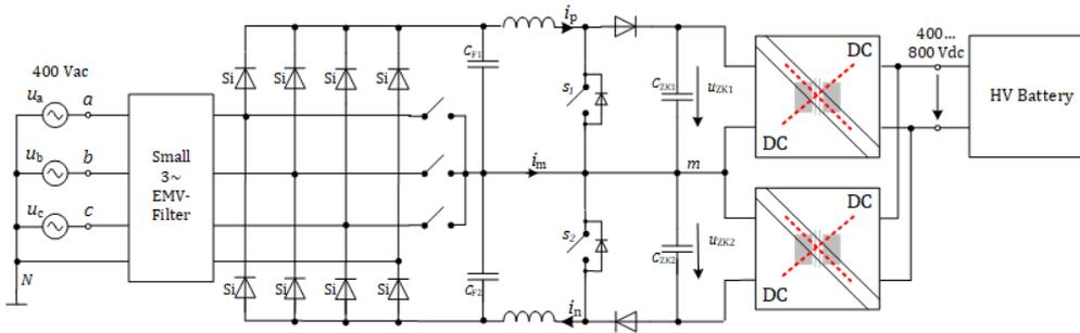
Circuit diagram for a low-common-mode, three-phase on-board charger. The low-common-mode PFC stage (three-phase and single-phase) allows for the omission of transformers in the DC-DC stage.
