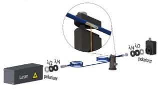
Device for precisely adjusting the linear polarization in a polarization-maintaining optical fiber. The magnification shows the heating element, typically a metallic wire, located at least along a portion of the optical fiber within the fiber sheath.
