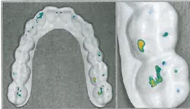
Device – prototype after intraoral use by volunteer and close-up of detail
