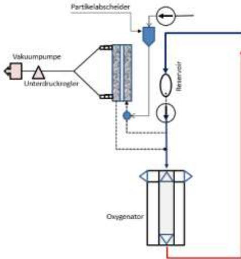
Experimental set-up in vitro circuit
